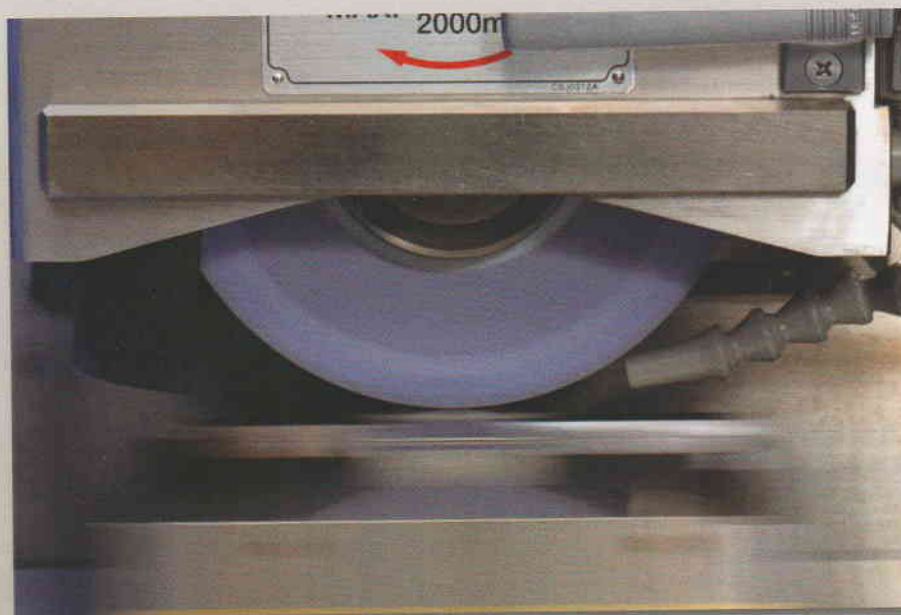
250 min -1 high reciprocation grinding
