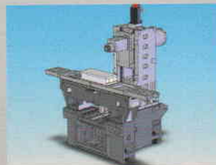
Three-face stand-alone column design
