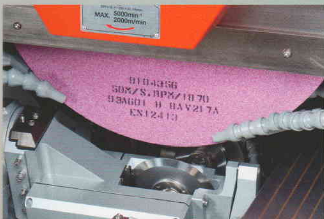
Swivel rotary dresser designed to suit high precision forming
