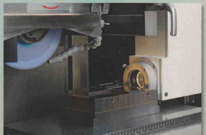
On-board measurement system that permits significant savings in work change time
