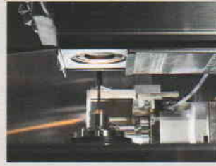
Automatic measurement with a CCD camera
