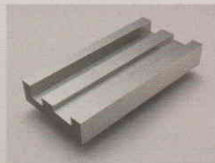
Unequal depth groove grinding
